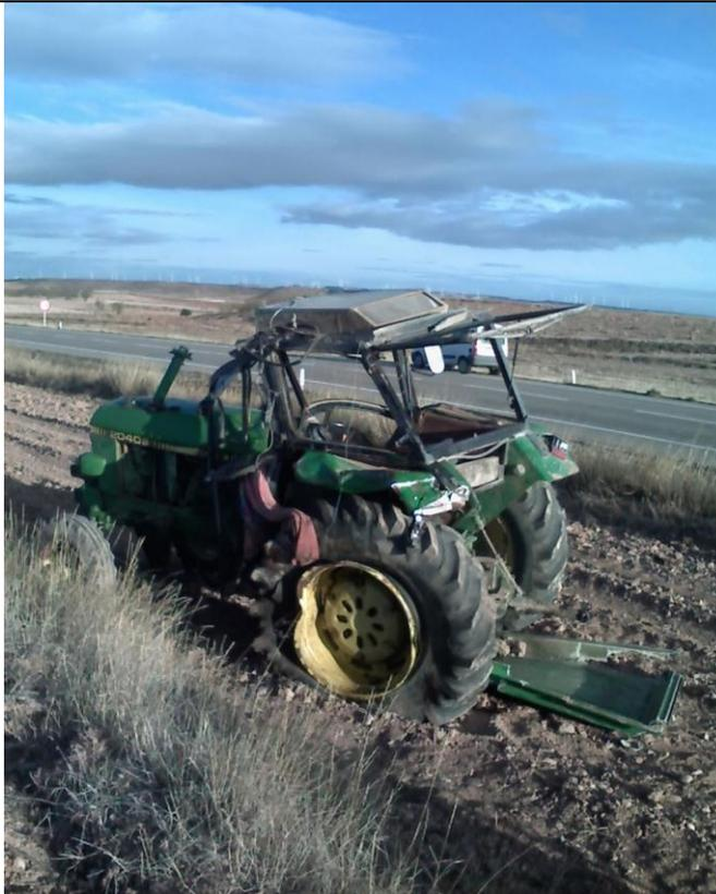
Picture of a tractor equipped with a cabin that successfully passed the new OECD Standard Codes for Official Testing.
